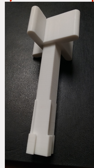
3D printed pinwheel to join optical separators and support the optical lattice
