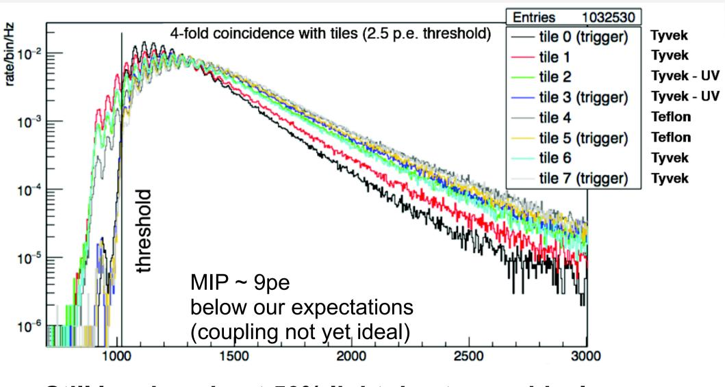
Still loosing about 50% light due to non ideal coupling of optical fiber and fiber-end mirror
