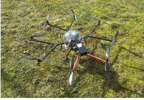
FIGURE 3. Octocopter used for the calibration measurements with mounted calibrated emitting antenna and GPS module.
