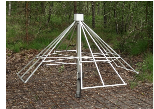
0.025 km 2 – 10 cabled antennas – compact phased array – External trigger
