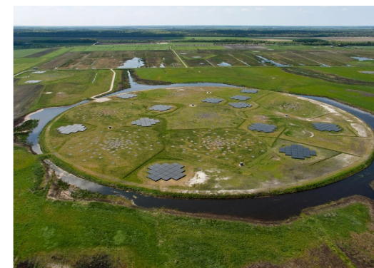
LOFAR superterp (Netherlands) – 21x96 antennas – \varnothing = 350 m
