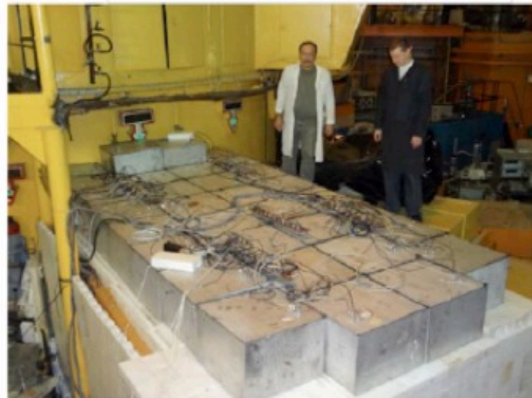
Installation of anticoincidence shielding from plastic scintillator 0.5x0.5x0.125 m 3 with PMT (32 pieces)
