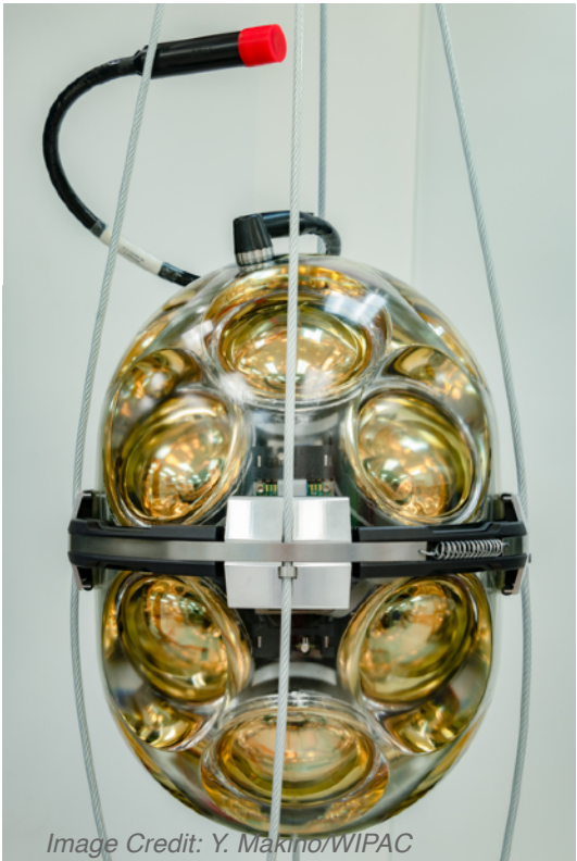
Gen2-DOM PMT segmentation with 4\pi angular coverage in an elongated vessel
