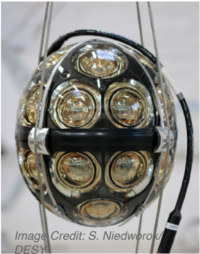
mDOM PMT segmentation with 4\pi angular coverage
