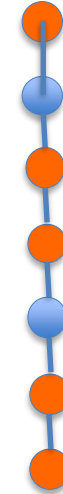
String trigger: N hits of M DOMs on a string in a time window
