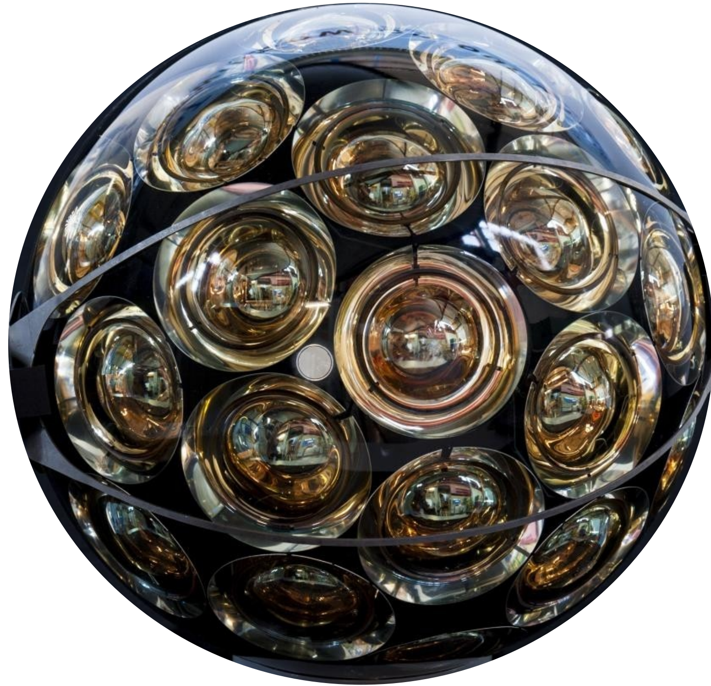
31 3" photo-multiplier tubes per Digital Optical Module (DOM)
