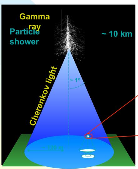
Cherenkov light image of particle shower in telescope camera
