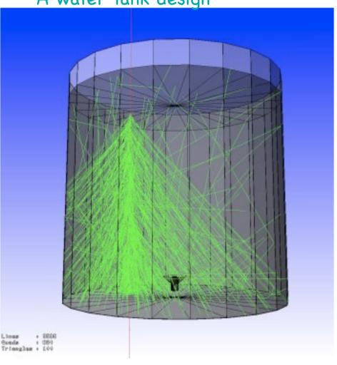
A 5 meter diameter tank as simulated in Geant4 for a single vertical muon. The number of photons are reduced by a factor of 50 for vizualization.
