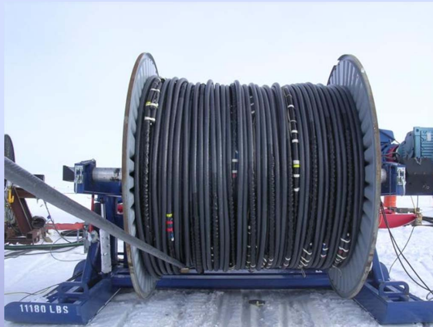
String cable 2500 m - Weight ~6 tons
