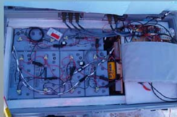
Electronics + batteries in vacuum enclosure
