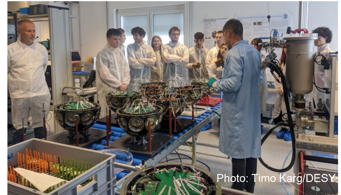
Upgrade: Optical module production at DESY, Zeuthen
