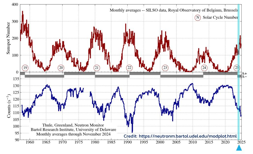
Monthly sunspot number (top) and neutron count rate from the Thule Neutron Monitor (bottom) from 1955 to 2024. The ARAON latitude survey (cyan vertical bar) occurred during the rising phase of Solar Cycle 25, coinciding with the reversal of the solar magnetic field polarity from A+ to A-.
