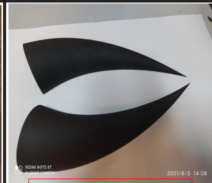
Teflon master mould to shape the absorbing coating
