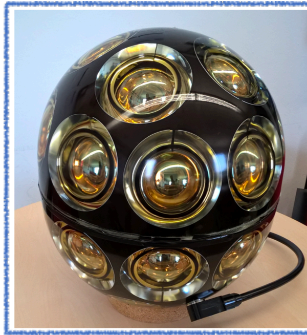
Directional information 24 x 3 inch PMT Diameter 36 cm
