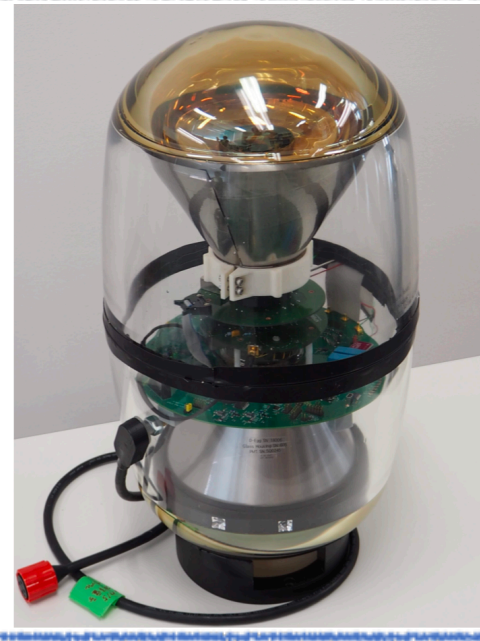
2 x 8 inch PMT Smaller diameter 30 cm
