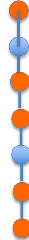
String trigger: N hits of M DOMs on a string in a time window
