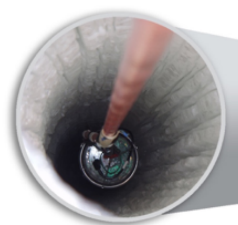
Digital Optical Module (DOM) 5,160 DOMs deployed in the ice
