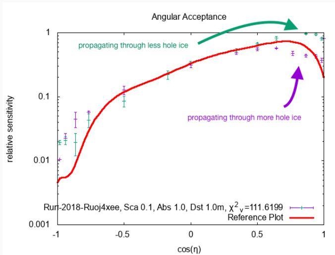
For each angle  $\eta \in [0; 2\pi[$ , shoot photons from planes onto the DOM and count hits.
