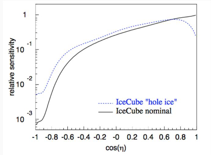
Angular acceptance *reference curves*. The nominal model is based on lab measurement, the hole ice curve on previous simulations.
