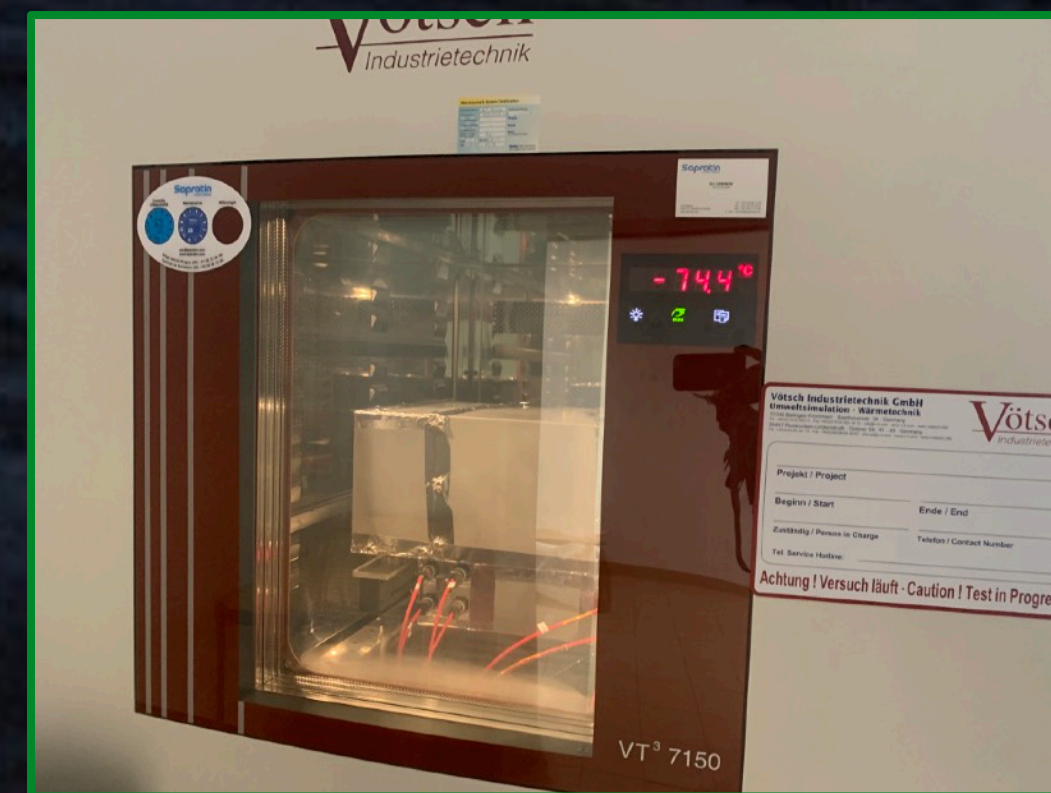
cold chamber tests @ -75°C
