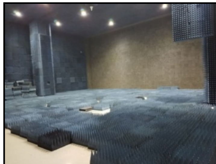
Antenna gain in-air (Anechoic chamber measurement)
