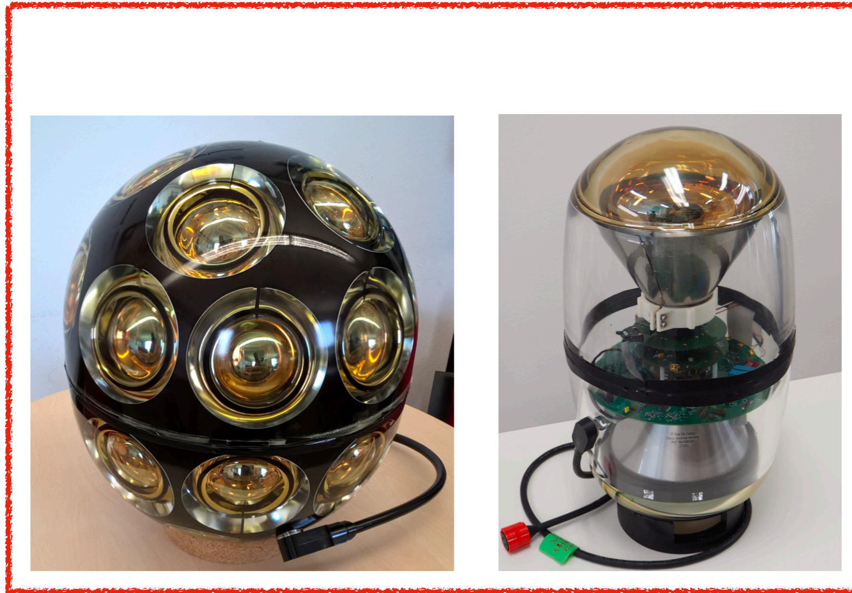
Directional information 24 x 3 inch PMT Diameter 36 cm
