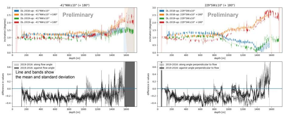
Measured inclination pattern is consistent throughout multiple runs and years Hole seems to be "straightening up", mostly at the top (?)
