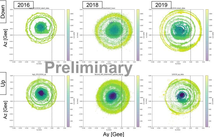
Accelerometer data is noisy probably due to tool rattling around the hole
