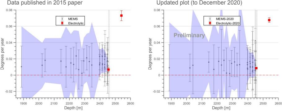
Long-term average inclination from two electrolytic (red) and 42 MEMS (gray) tilt sensors. The electrolytics are at 2455 m (86% ice sheet depth) and 2540 m (90%). Error bars show standard deviation from trend and the shaded area is the MEMS 95% confidence. (Right) Newer data over a longer baseline; note that new MEMS data are unprocessed.
