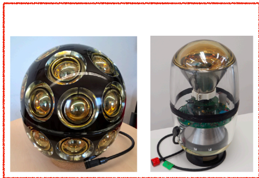
Directional information 24 x 3 inch PMT Diameter 36 cm
