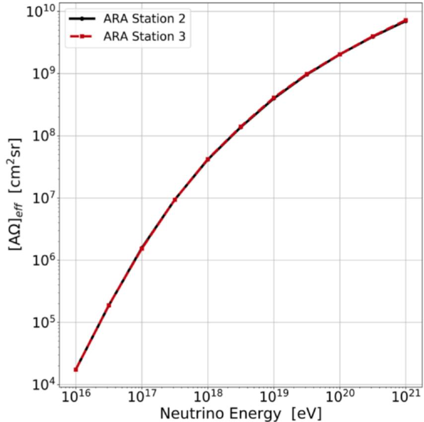
Fig. 3. The simulated trigger-level effective area-steradian ( $[A\Omega]_{eff}$ ) for ARA stations A2 and A3, averaged across configurations.
