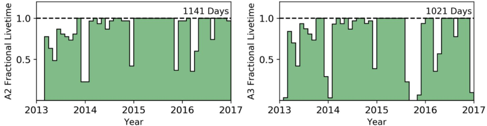
Fig. 2. Fractional livetimes for A2 (left) and A3 (right) from deployment in 2013 through the end of the analysis period in 2016. From the 4 years of deployment, roughly 3 years are analyzable due to intermittent downtimes.
