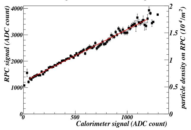
→ Linearity up to ≈ 2 · 10<sup>4</sup> particle/m<sup>2</sup>
