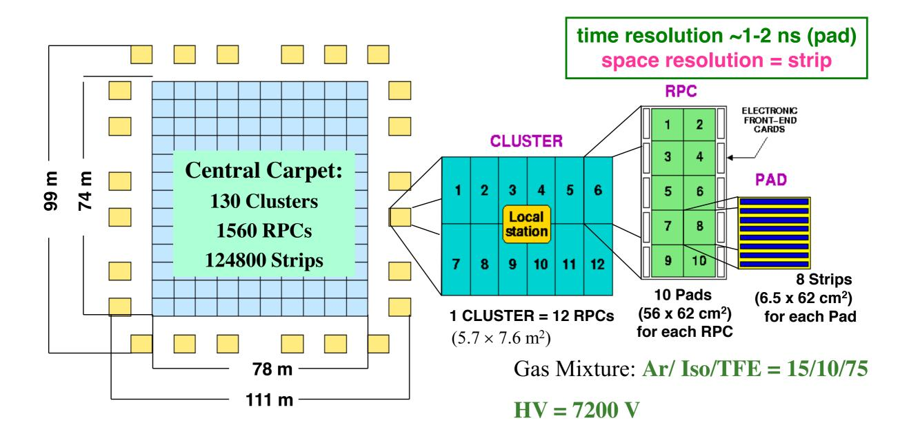
Single layer of Resistive Plate Chambers (RPCs) with a full coverage (92% active surface) of a large area (5600 m<sup>2</sup>) + sampling guard ring (6700 m<sup>2</sup> in total)
