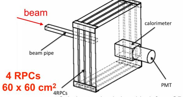
Calorimeter: lead glass block from OPAL, PMT a Hamamatsu R2238.
