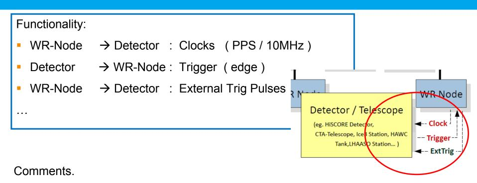
(1) TriggerTimes are generated both on detector and WR-Node for each event.
