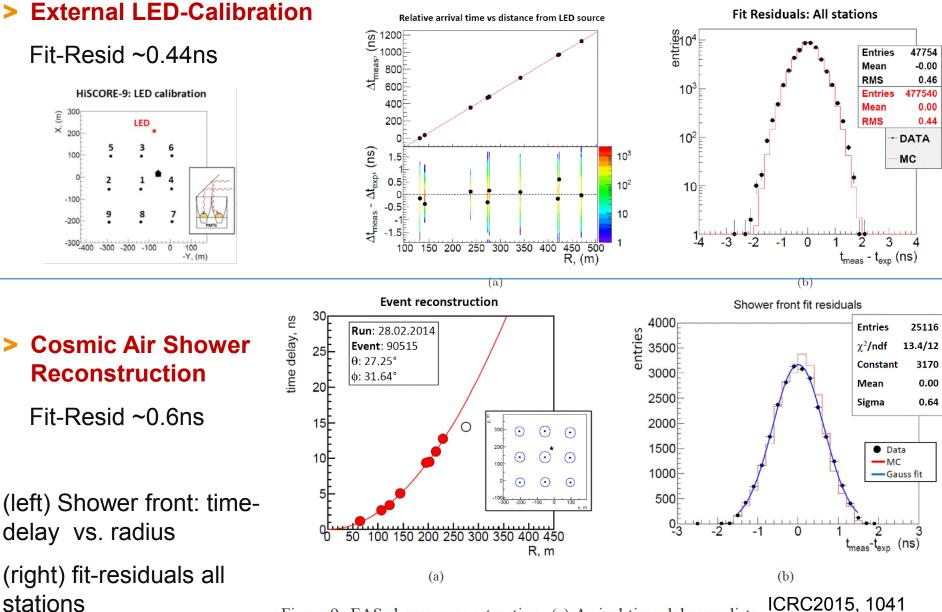
Figure 9: EAS shower reconstruction. (a) Arrival time delay vs dista
