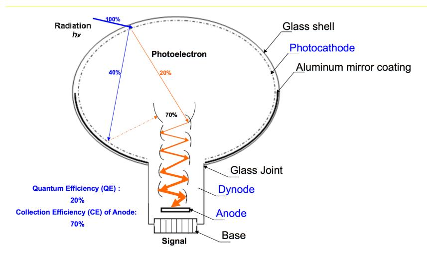
Photon Detection Efficiency (PE)= QE<sub>Trans</sub> \* CE = 20% \* 70% = 14%
